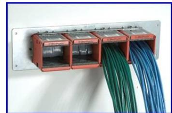
For example, the typical column pressure occurring in an enclosure with an FM200™ system would be around 10-15 Pa. At these pressures, an empty Series 22 device will add approximately .08 in<sup>2</sup> (0.50 cm<sup>2</sup>) leakage to the enclosure while a fully loaded Series 22 device will add approximately 0.09 in<sup>2</sup> (0.58 cm<sup>2</sup>).
